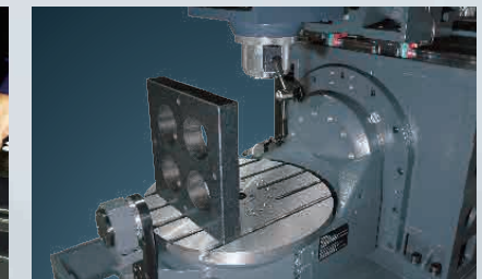
Measurement of linear axes perpendicularity on 5-axis machine
