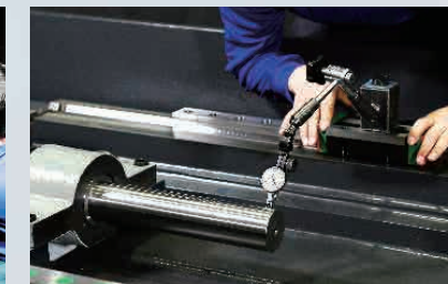
Parallelism measurement between ball screw and linear guideway
