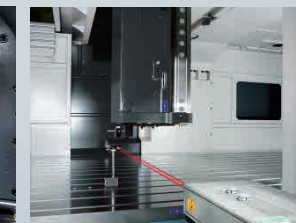
Laser detection of accuracy
