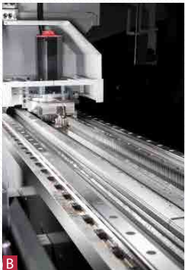
Adjustable Crossbeam Structure AWEA patented design has successfully overcome the physical limits, minimizing the deformation caused by the weight of the 7,000 mm super wide cross beam, thus ensuring optimal machining accuracy.
