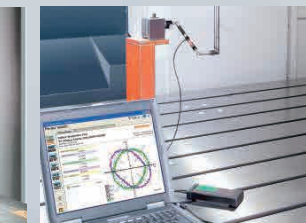
Ball bar detection for 3 axes
