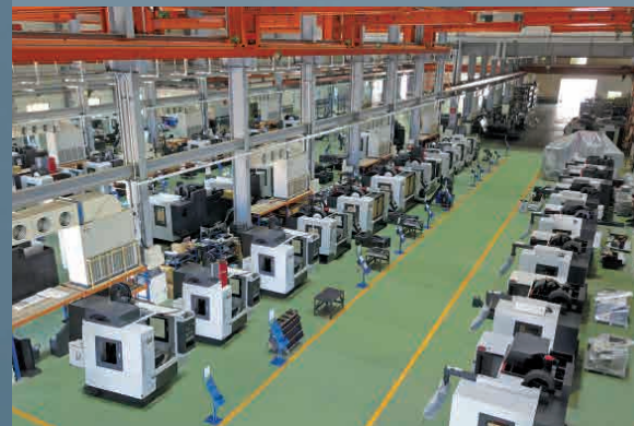
VMC production line of the new Chiayi factory
