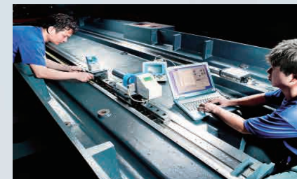
Straightness check for linear guide ways
